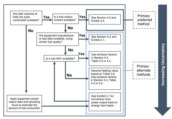
Figure 3.5. Example of GHG "decision tree" for combustion sources (based on API 2009)
