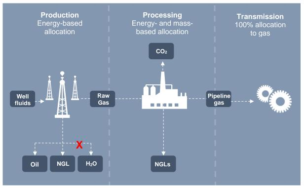
Figure 10.1. Block diagram for typical gas production, processing, and transmission
