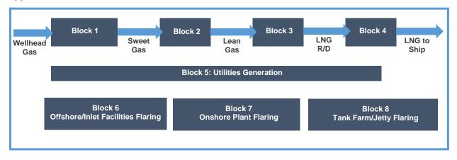
Figure 10.2. Example process block breakdown for an LNG plant
