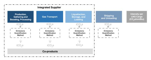
Figure 3.1. Representation of LNG value chain with co-product allocation
