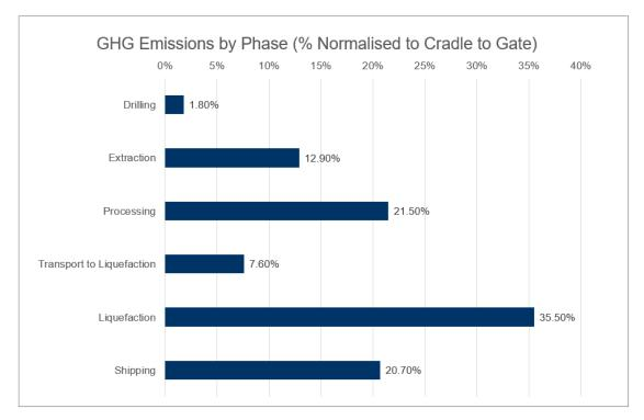
Figure 2.3.3. Proportion of GHG emissions by stage of the LNG production chain – normalised to cradle to gate (adapted from PACE Global, 2015 full life cycle assessment)
